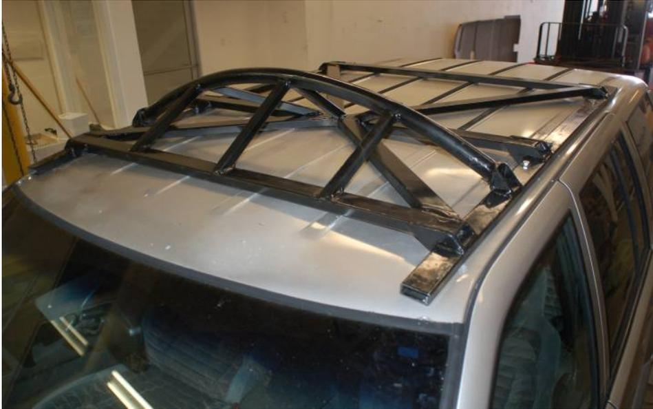
Figure 15. Prototype RDMD fitted to roof of low strength (1993) vehicle.
