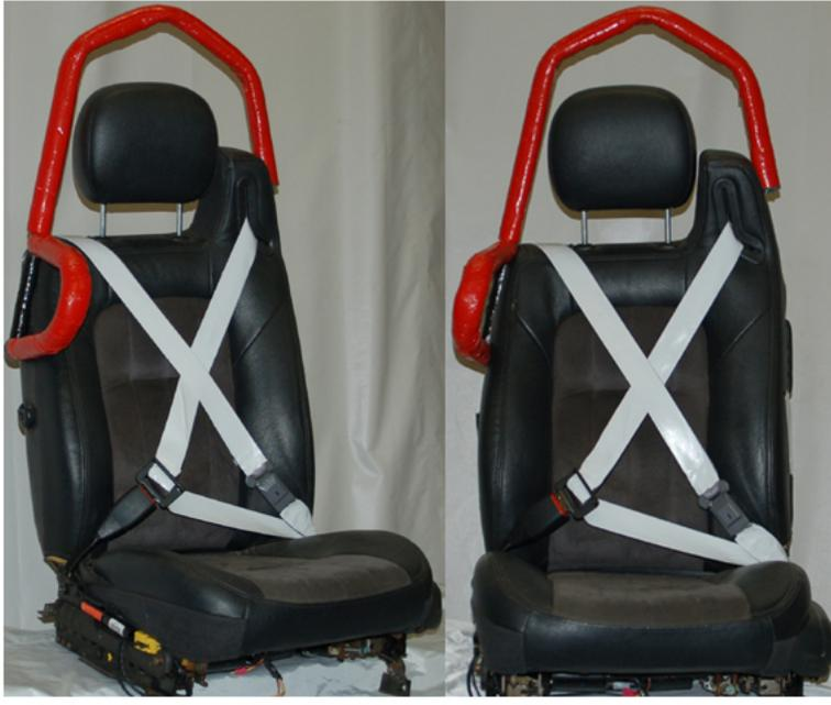
Figure 33. Prototype All-Belts-to-Seats Occupant Protection System.
