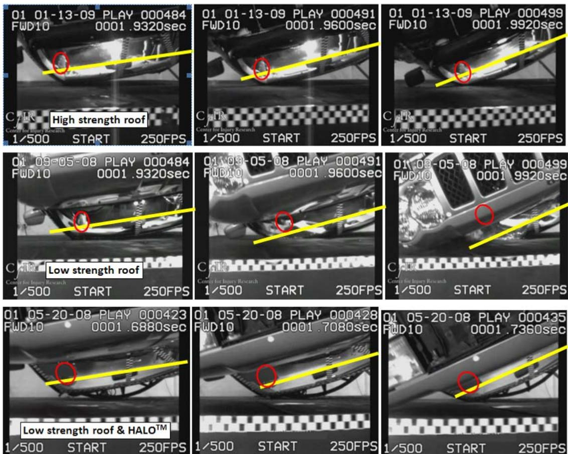
Figure 18. Top row: high strength roof; Middle row: low strength roof; Bottom row: low strength roof with RDMD.
