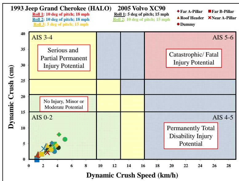
Figure 28. Final RDMD HALO design compared to Volvo XC90 Performance
