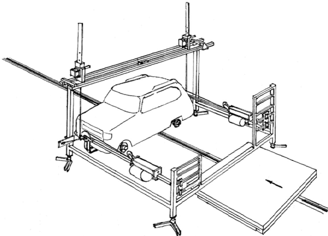
**Figure 5:** Top: Concept model of UNSW JRS rig.
