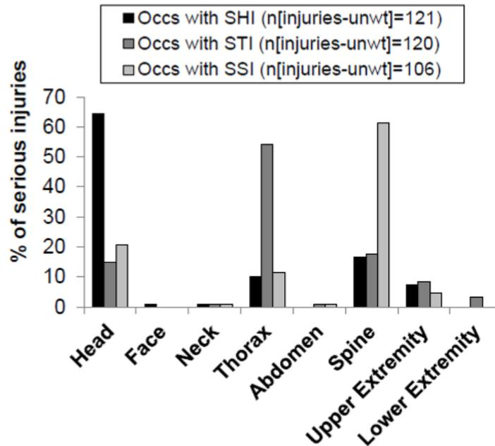
**Figure 2:** Distribution of occupants with serious injuries AIS 3+ by body region for contained, restrained occupants greater than 16 years old in pure, trip-over rollovers (after Mattos et al [24]).
