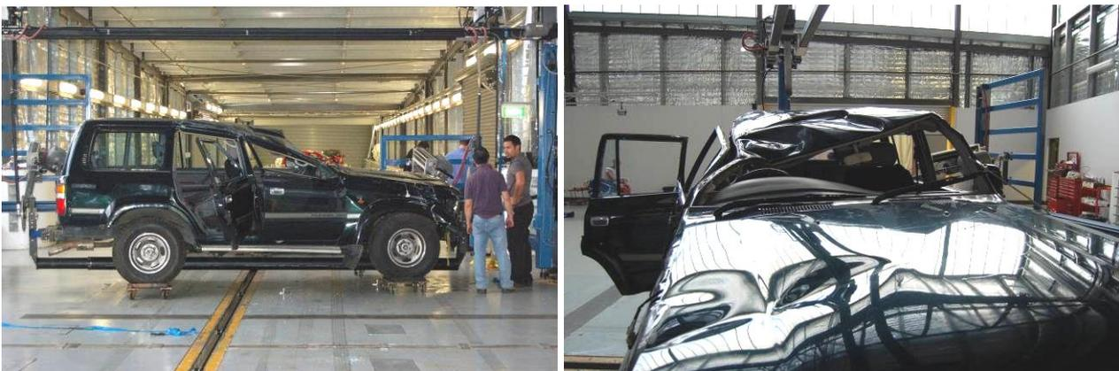
**Figure 7:** Damage profile of the 1998 Toyota Land Cruiser after one roll.
