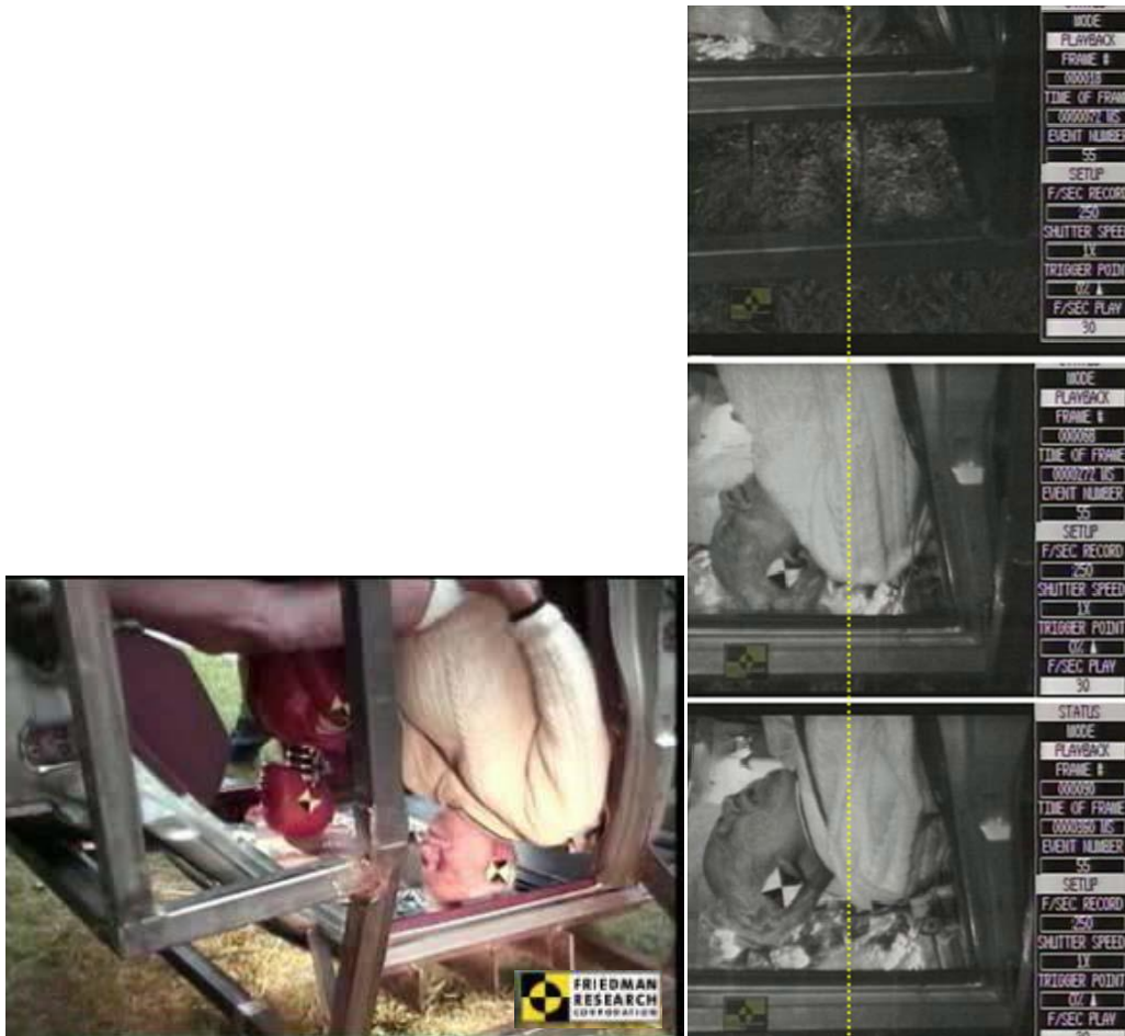
Figure 6. (Left) Dummy and human in drop test fixture. (Right) High speed video frames of 30-cm drop test
