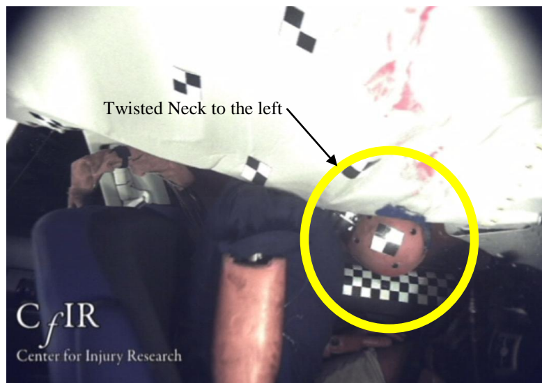
Figure 3. Scion xB bent and twisted neck
