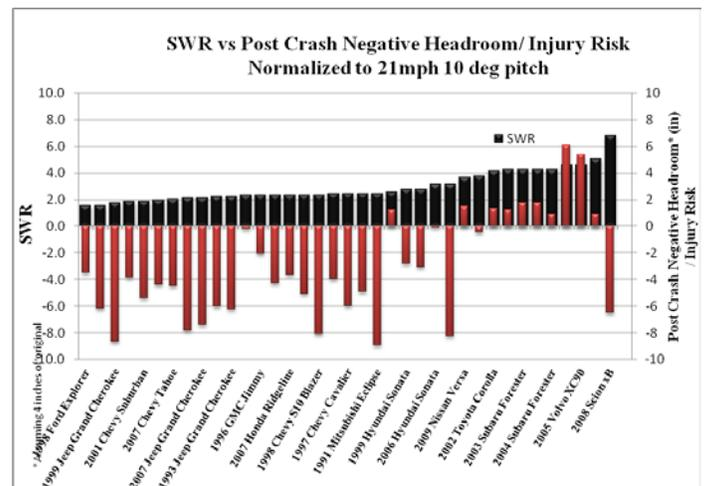
Figure 3. Post-crash positive and negative headroom in order of ascending vehicle SWR.
