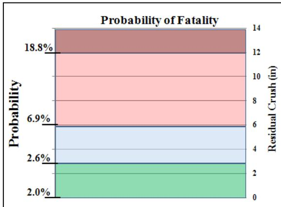
Figure 4. A fatal probability function vs. residual crush.
