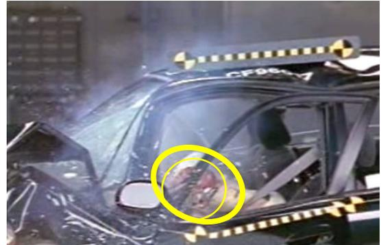
Figure 12. IIHS 1996 Hyundai Sonata (40%) offset frontal test at 40 mph at maximum head excursion.
