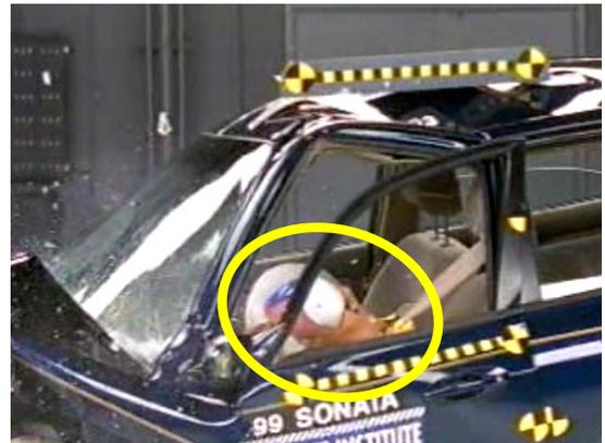
Figure 13. IIHS 1999 Hyundai Sonata (40%) offset frontal test at 40 mph at maximum head excursion.
