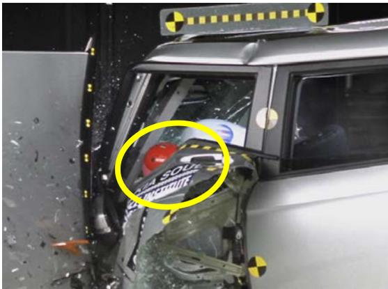
Figure 10. IIHS 2012 Kia Soul small (25%) overlap test at 40 mph at maximum head excursion.
