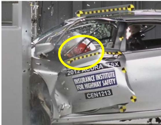
Figure 11. IIHS 2012 Acura TSX small (25%) overlap test at 40 mph at maximum head excursion.
