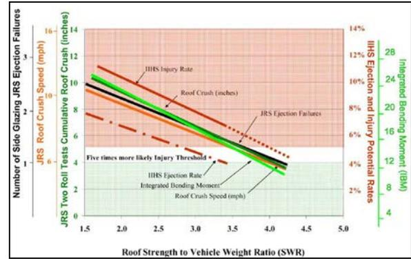
Figure 2. Composite plot of injury measures showing rate reduction with increasing vehicle SWR.
