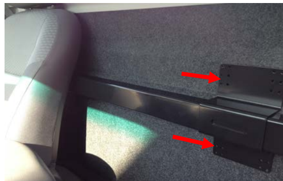
Figure 11. Single-Cab HALO™ B-Pillar Cross-member
