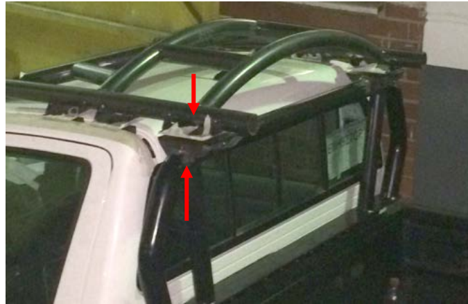
Figure 12. HALO™ roof top mounts to rear roll hoop
