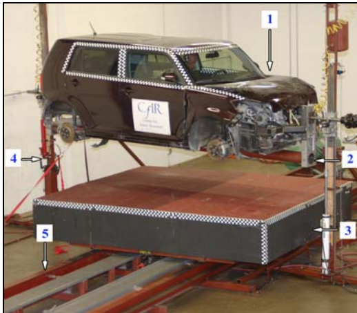
Figure 11. Key Components of The JRS: 1) Vehicle, 2) Cradle/Spit Mount, 3) Moving Roadbed, 4) Support Towers, 5) Coupled Pneumatic Roadbed Propulsion and Roll Drive
