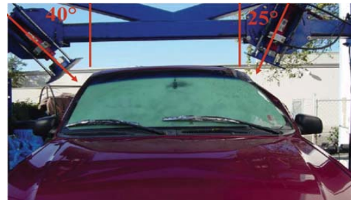
Figure 4. Vehicle in M216 test fixture indicating 25° and 40° platen angles.
