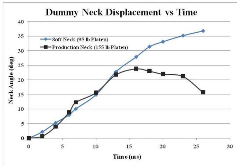
**Figure 4. Pendulum Test.** Bending angle as a function of time with different platen weights.
