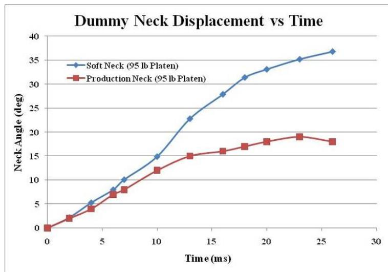
**Figure 3. Pendulum Test.** Bending angle as a function of time with 43 kg (95 lb) platen
