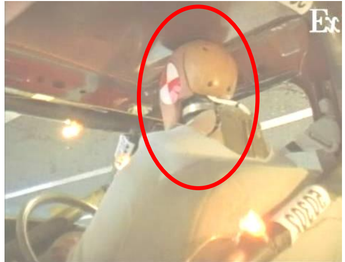
Figure 3. 1998 Crown Victoria (low severity rollcage 50302) max roof crush
