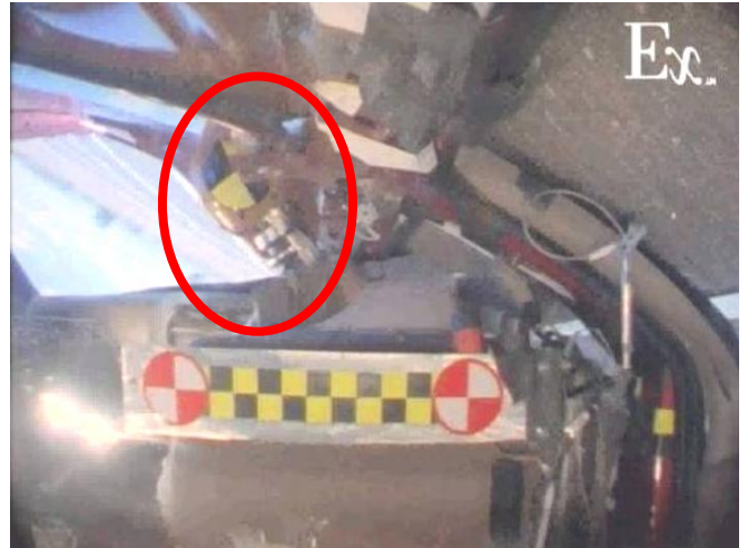
Figure 8. 1996 Chevrolet Blazer (low severity 41703) max roof crush
