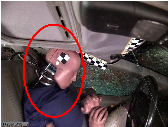
Figure 10. 1998 Ford Explorer (Production Roll 1) max roof crush
