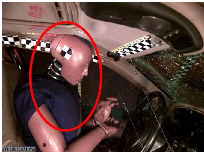
Figure 13. 1998 Ford Explorer (Reinforced Roll 2) max roof crush
