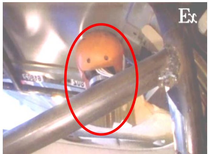
Figure 5. 1998 Crown Victoria (med. severity rollcage 61802) max roof crush
