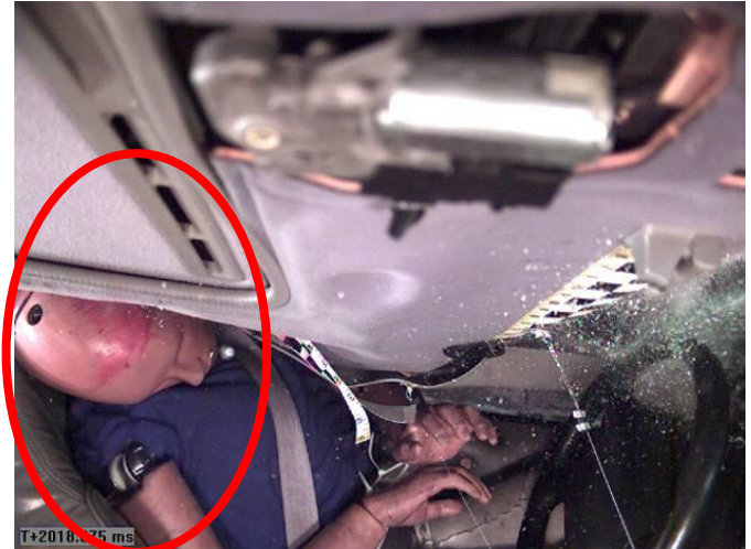
Figure 11. 1998 Ford Explorer (Production Roll 2) max roof crush
