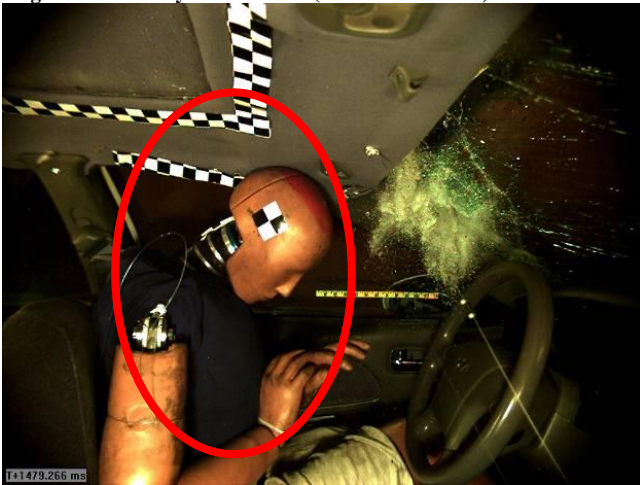
Figure 15. 1999 Hyundai Sonata (Reinforced Roll 1) max roof crush
