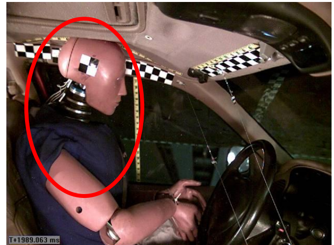
Figure 12. 1998 Ford Explorer (Reinforced Roll 1) max roof crush
