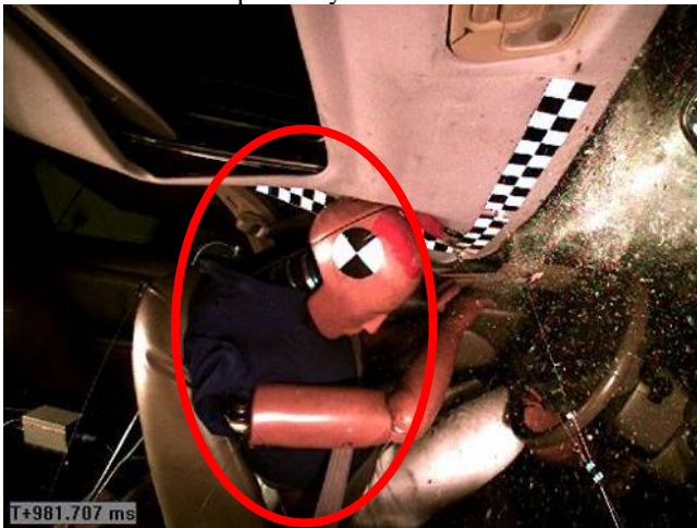
Figure 14. 1999 Hyundai Sonata (Production Roll 1) max roof crush
