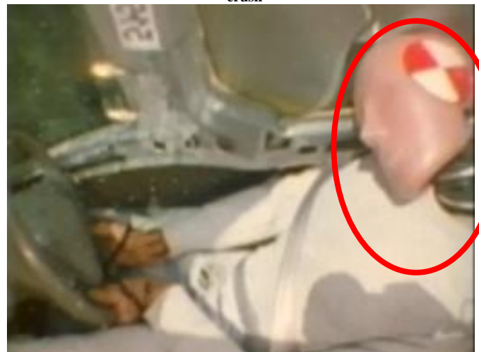
Figure 4. 1998 Crown Victoria (low severity 51502) max roof crush
