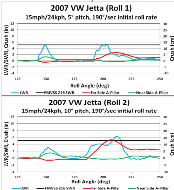
Figure 13. Jetta Roof Crush vs. Roll Angle.
