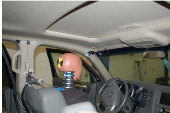
**Figure 5. String Potentiometers to A Pillar**
