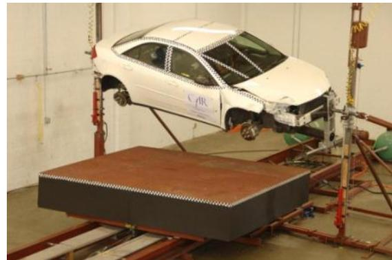
**Figure 1. Jordan Rollover System (JRS) Test Rig.**
