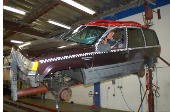
Figure 34. JGC with HALO™ After 2 Test Rolls.
