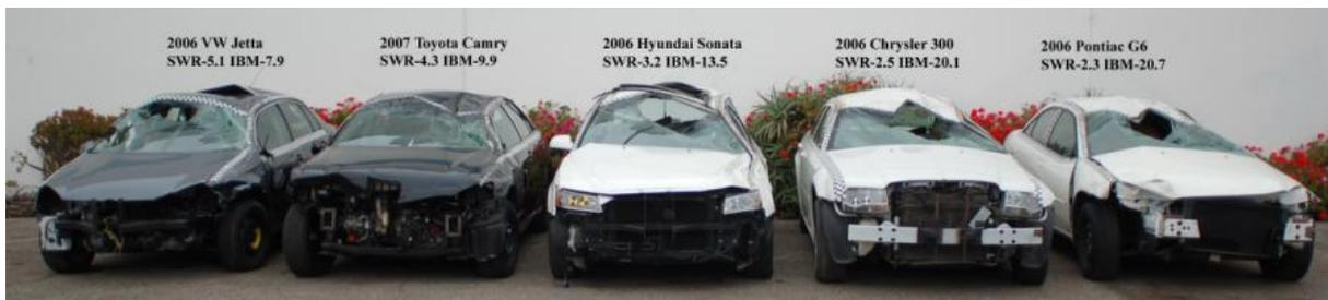
**Figure 6. JRS Post Test Two Roll 5 Passenger Vehicles.**
