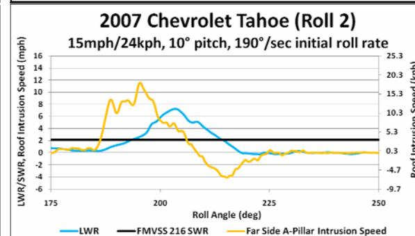
Figure 20. Tahoe Peak Roof Intrusion Speed.
