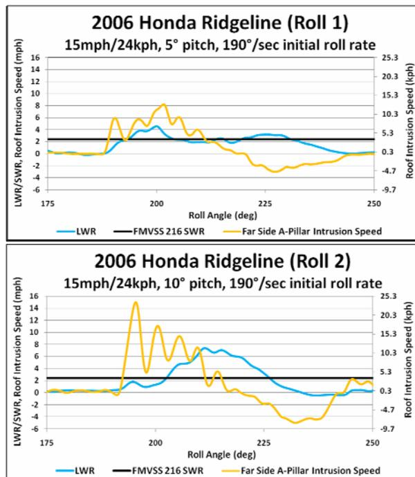
Figure 12. Ridgeline Peak Roof Intrusion Speed.
