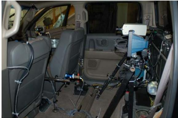
**Figure 4. Vehicle Interior String Potentiometers**
