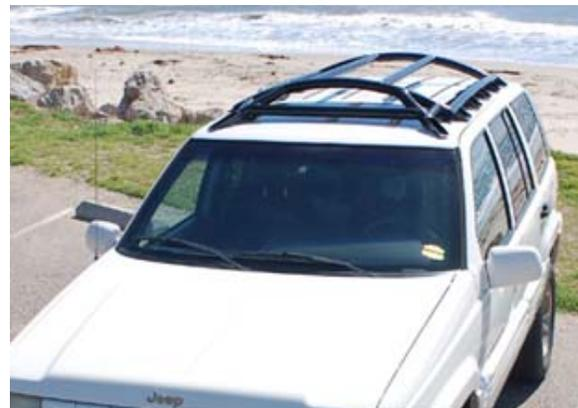
**Figure 28. HALO™ Roof Damage Minimization Device**
