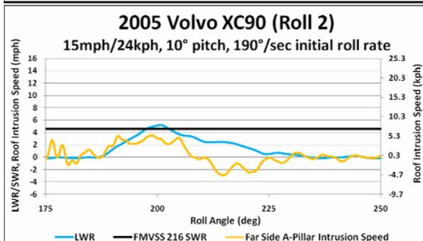
Figure 19. XC90 Peak Roof Intrusion Speed.
