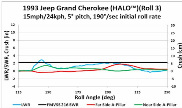
Figure 41. JGC w/HALO™ Roll 3 Roof Crush
